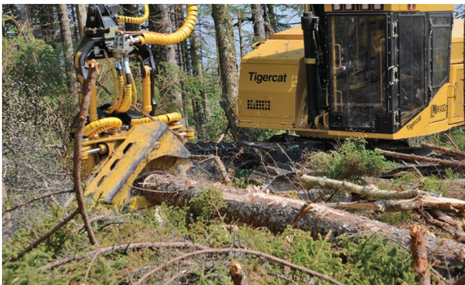
Tigercat's 570 is a high performance harvesting head ideally suited to the Tigercat H845 series carrier.
