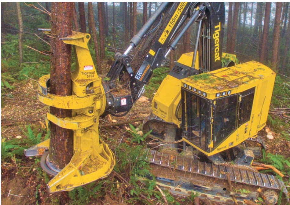
The LX830D model feller buncher is designed for steep terrain and features a closed loop track system that allows for speed and superior performance.
