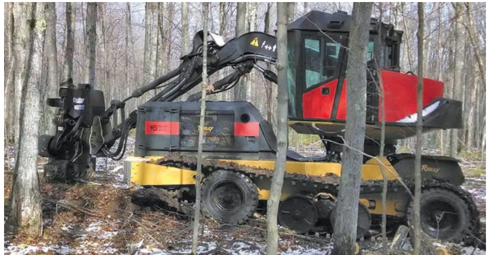
The E-Clips® has a Risley Flex-Trac® high-speed track system like an Army tank, with a rubber-bushed, steel-pad configuration. “Speed, along with traction and terrain capabilities, mean this machine can really climb and, at speeds above six mph, can compensate easily when a track goes over a rock,” said Reg Isley.
